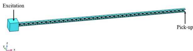
Fig. 6 A finitely long PCSB containing 20 RVEs under the base excitation
